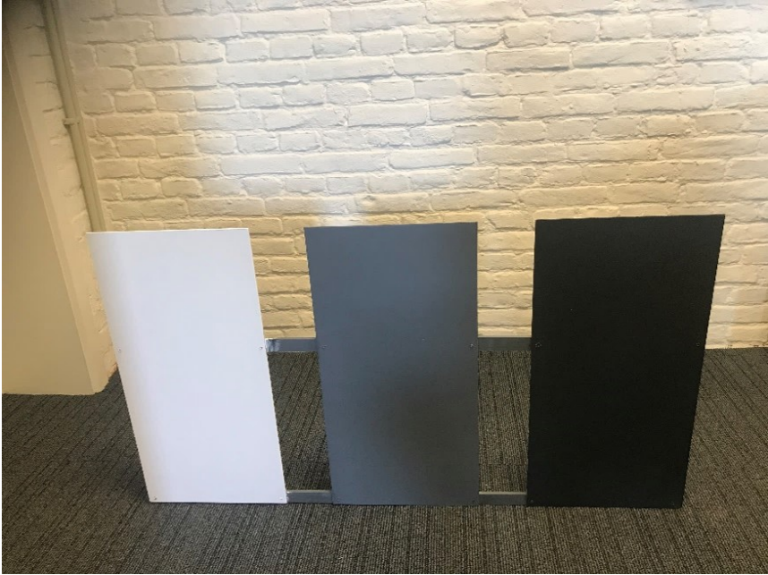
Figure 6.3: photograph of the test plates painted white, gray, and black.
