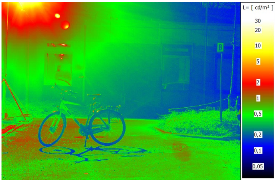
Figure 6.9: luminance image of the KU Leuven bike positioned at 10 m from the light mast using counterbeam illumination. The luminance is color coded by the color bar on a logarithmic scale.
