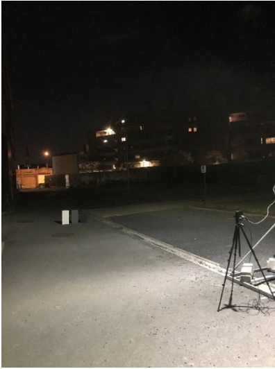
Figure 6.4: photograph of the experimental setup including the LMK5-5 Color luminance camera.
