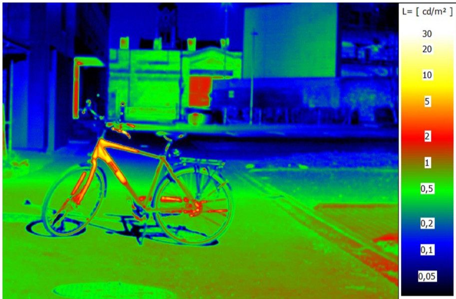
Figure 6.8: luminance image of the bike positioned at 10 m from the light mast using probeam illumination. The luminance is color coded by the color bar on a logarithmic scale.
