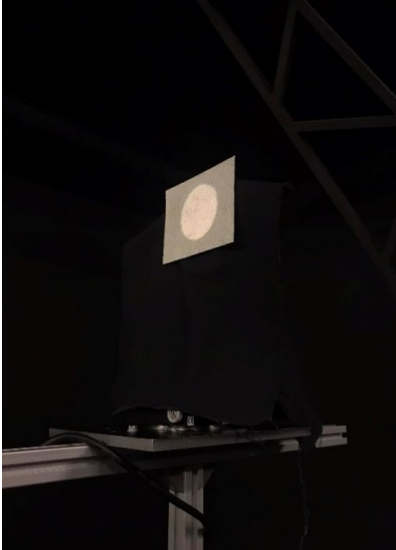
Figure 4.2: A photograph of the sample and sample holder, showing the circular light spot with a diameter of 7.5 cm on the test sample at perpendicular incidence.
