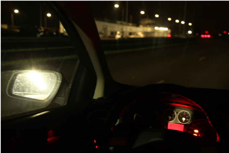
Figure 6.20: photograph of the glare experienced in the left side mirror from the driver's position in the car with the Probeam prototype installation.
