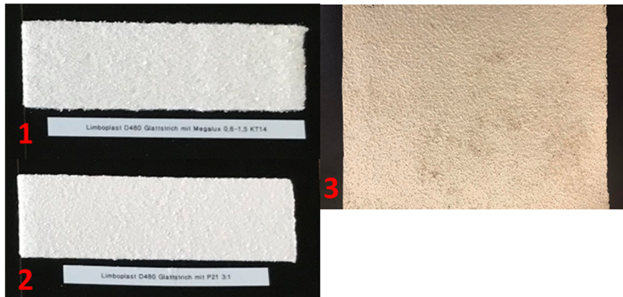
Fig. 3. Photographs taken from the three test samples: (1) SWARCO Limboplast D480 with Megalux 0.6-1.5 KT14, (2) SWARCO Limboplast D480 with P21 3:1, and (3) 3M Stamark A650.
