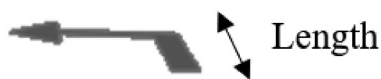
Fig. 4. Image of a road marking arrow with an indication of its length.
